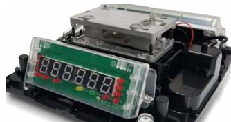
Sealed & Protected PCB
